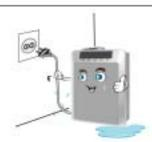
Do not use your ionizer at voltages other than specified (AC 110V FOR USA). Use a GFI outlet. Do not plug in your ionizer where it will exceed the rating of
